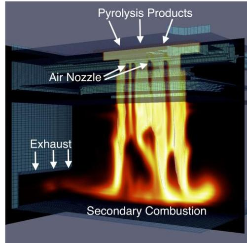
The image at right is from a recent analysis performed by Professor DesJardin in support of this project. It depicts turbulent combustion of pyrolysis products mixed with fresh air provided by the inlet small inlet nozzles of the boiler.
